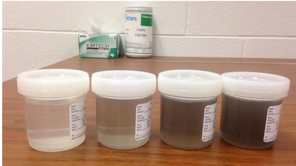
Figure 11: phantom solutions of Luxsil microspheres
